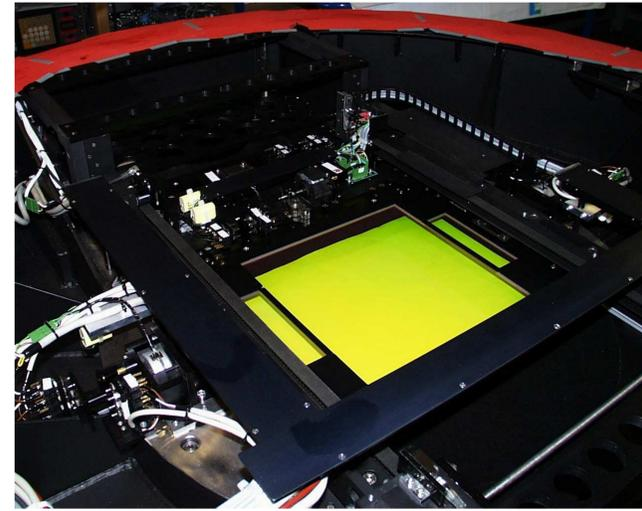
Figure 4: The  $r'$  filter in the light path (main field of view  $268 \times 268$  mm). On the right and left side of the science filter the auxiliary filters for guiding and image analysis are visible. The total mass of the filter including frame is 6kg. Note that the shutter was not mounted when the picture was taken.
