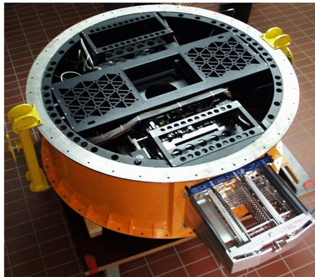
Figure 3: The 1.5 m diameter housing structure with integrated shutter (structure going from left to right) and storage magazines for filters (upper and lower part). The filter loading platform is attached to the housing. Each magazine can be filled with up to 6 filters which are large and heavy: when fully loaded with 12 filters, the instrument will contain 40 kg of filter glass alone! During the filter exchange process about 17kg are moved (mass of 2 filters and the carriage).
