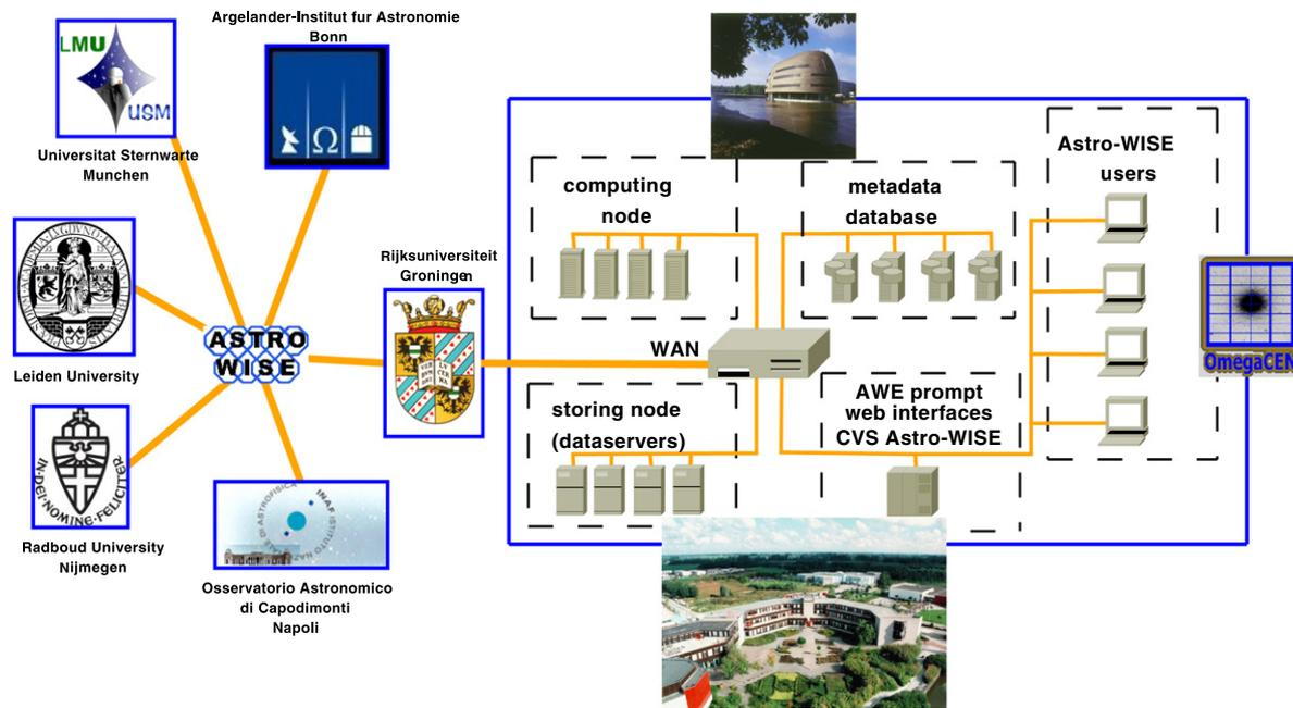
**Fig. 3.** Typical architecture of an Astro-WISE site in full mode (data storage node, computing node, web interfaces, CLI and version control system). The Rijkuniversiteit Groningen Astro-WISE node is shown (the computing node and metadata database are hosted by Donald Smits Center for Information Technology—CIT, top picture, the other elements are hosted by Kapteyn Astronomical Institute/OmegaCEN, bottom picture), sites of other participants have similar structure.
