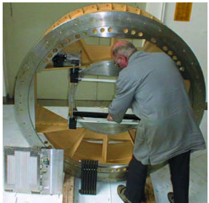
Figure 3: The 1.5-m diameter housing structure during a test assembly of the main units: the two storage magazines (to be inserted into the big shaft at left and hidden right), the filter exchange unit with the exchange carriage and a 420 \times 320 \text{ mm}^2 opaque, aluminium 'filter' (at the bottom left).
