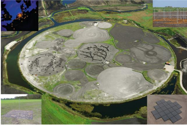
**Fig. 1.** The core of the LOFAR telescope (central photo) with low-frequency and high frequency antennas (lower corner pictures) and low-frequency antenna field (upper right corner). The final configuration of LOFAR antenna fields in the full deployment mode is shown in the picture in the left upper corner (with the core in the center and Dutch national and international stations).
