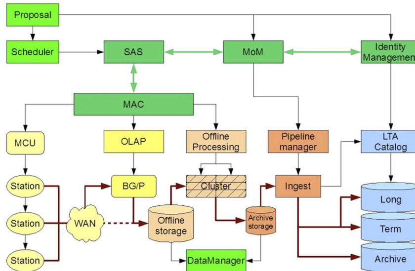
Fig. 2. LOFAR raw data processing and data ingest.
