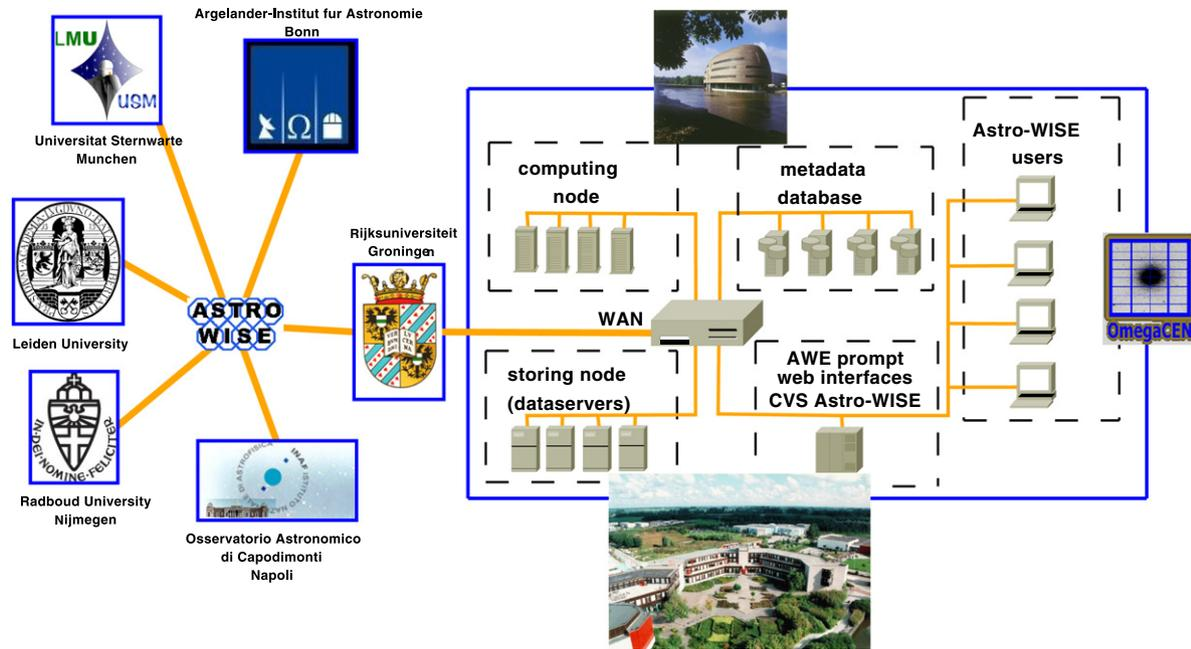
**Fig. 3.** Typical architecture of an Astro-WISE site in full mode (data storage node, computing node, web interfaces, CLI and version control system). The Rijksuniversiteit Groningen Astro-WISE node is shown (the computing node and metadata database are hosted by Donald Smits Center for Information Technology—CIT, top picture, the other elements are hosted by Kapteyn Astronomical Institute/OmegaCEN, bottom picture), sites of other participants have similar structure.
