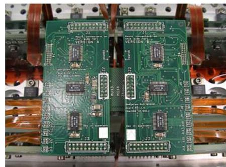
Figure 23: CCD head integrated dual multiplexer
