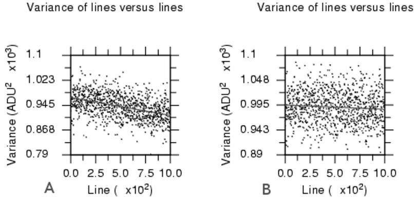
Figure 1. Image A and B show the plot  $(i, \sigma_a^2(i))$  at different CTEs with the best fit line in red. In A, the CTE is 0.999970 and in B, 0.999996. These plots have been done with simulated data. The dimensions of the images are 1k x 1k. The number of electrons in the images is 1000 plus a Poisson noise. The CTE is applied after. Similar pattern are observed with real data. In the x-axis, the line count increases away from the readout register.
